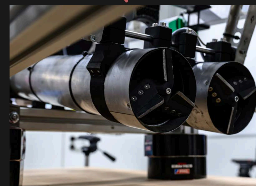
Fig.1 Excavating heads integrated into the rover's digging module
